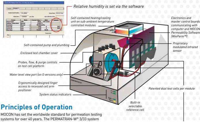
MOCON has set the worldwide standard for permeation testing systems for over 40 years. The PERMATRAN-W® 3/33 system uses a patented modulated infrared sensor to detect water vapor transmission through both flat materials and packages. This high performance sensor provides parts-per-million sensitivity.
