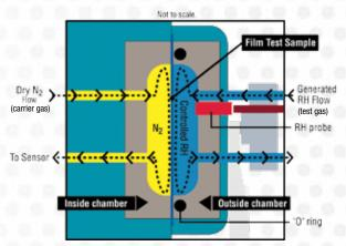
The G Plus versions of this system allow you to simultaneously condition and test materials over a wide range of temperature and relative humidity conditions similar to a package's actual storage environment. The film test cell in the PERMATRAN-W® 3/33 module incorporates RH probes in both cells to allow for control of the generated RH levels.
